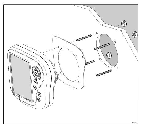
Figure 2-4: DS400/500 Flush Mounting Arrangement
